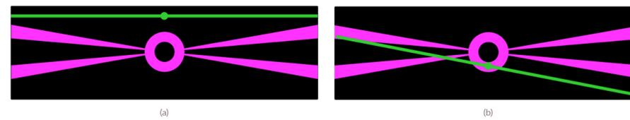
Bowtie heads-up display (magenta polygon) which participants controlled during the compensatory tracking tasks (a) Single-axis Condition, (b) Multi-axis Condition [9]
